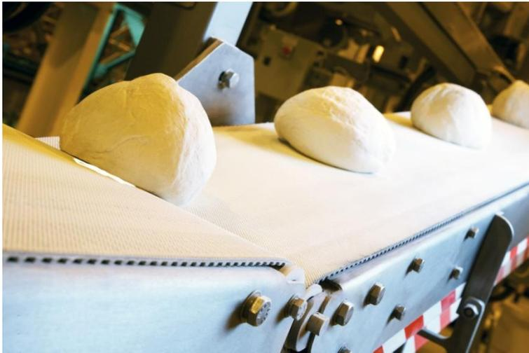
BMG's extensive range of Ammeraal Beltech belts includes low stretch Ziplink belts, designed for quick installation and replacement in diverse industries, including food and packaging sectors.
