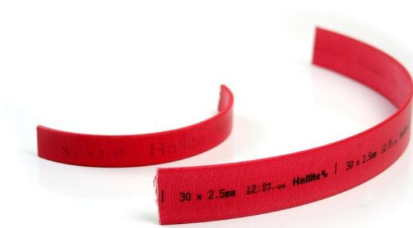
The material's design incorporates micro-indentations on the bearing strip's surface to trap fluid and provide built-in lubrication to the bearing. The bearing strip is manufactured using a woven fabric reinforced polyester resin material that is compatible with different fluids, including mineral oils, water based fluids and phosphate esters.
